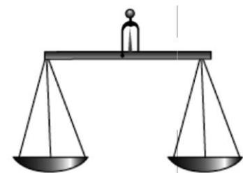
Figure: A beam balance
