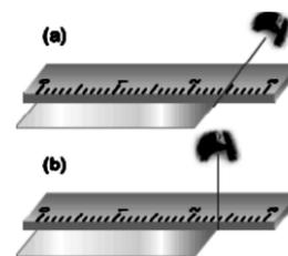
(a) Wrong position of the eye to note the reading.
